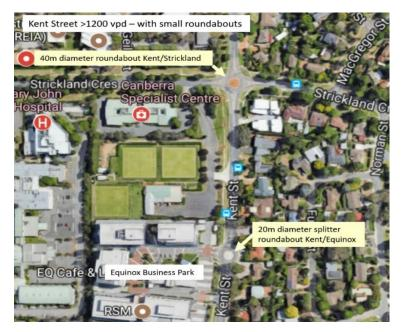
For comparison there is an equivalent intersection at the junction of the first stage of the Equinox Business Park with Kent Street in West Deakin in 2011, has just a small splitter roundabout. Kent Street carries some 12267 vpd (2014) and the Equinox is a large Business Park, which became fully operational in 2015/14, has a Gross Floor Area of commercial space of 25,000 sq m and underground paid parking for 512 vehicles.
